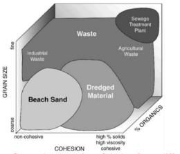
Figure I – General properties of sludge from different sources
