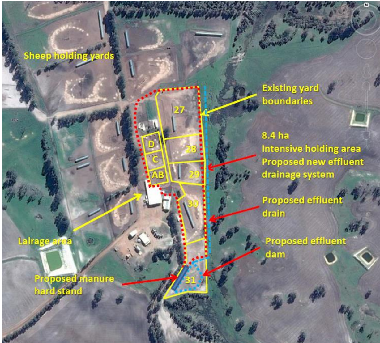
Figure 2: Location of intensive holding area and proposed effluent drainage system and evaporation dam
