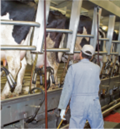
Sloped stainless steel pans — conform to natural cow shape.
