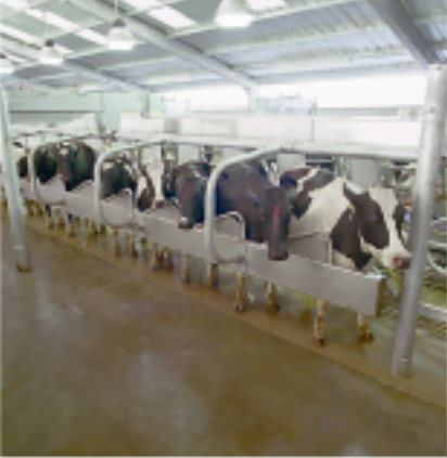
Individual cow positioning guide — brings all sizes of cows into correct milking position.
