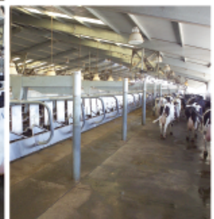
Rapid release exit — all cows leave quickly from the front to allow faster cow throughput.
