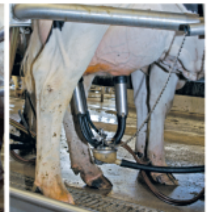
Chain take off system — integrated into the butt pan with smooth, positive vacuum shut-off combined with auto returning hose support arm.
