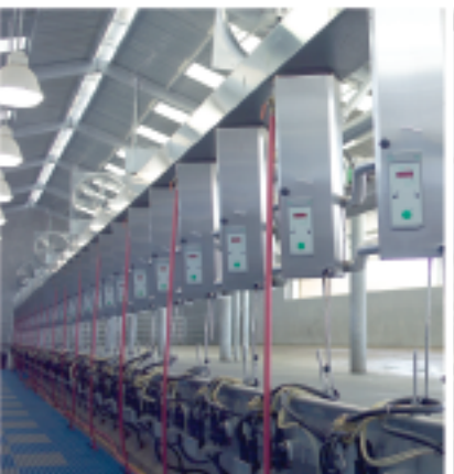
Metatron 21 milk meters — integrated herd management system monitors milking performance, cow health and milk quality.
