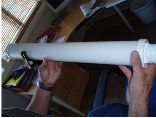
Figure 9.30 These plastic tubes are used for distributing air beneath trickle filters (see 9.31).
