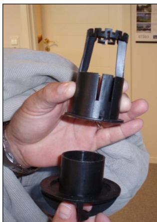
Figure 6.1. Water dispersion nozzle recommended for use instead of dispersion plates.
