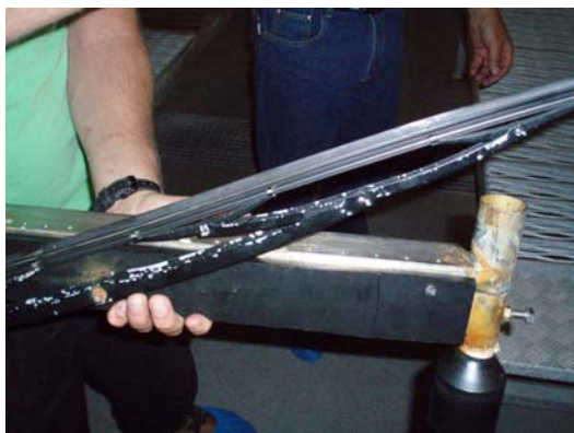
Figure 9.10 Part of the automatic tank cleaning system for the larval rearing tanks. The wiper blade attaches to a central rotating shaft. See 9.11
