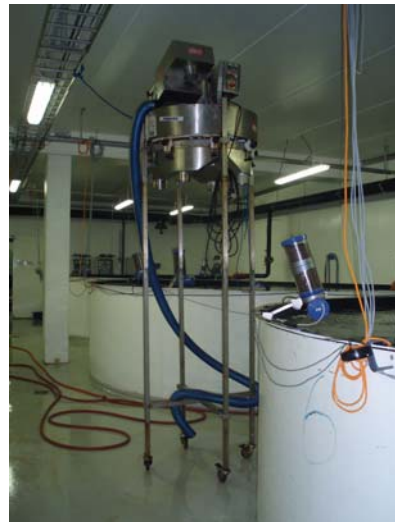
Figure 9.23 They had recently purchased a new Vaki brand grader. Although efficient we have doubts on how practical it is to operate. It appears to be very 'top heavy' and potentially unstable.
