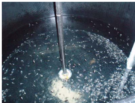
Figure 9.11 The inside of a halibut culture tank. The rod in the centre of the tank is the shaft to which the cleaning blade attaches. It is driven by a motor positioned underneath the tank.
