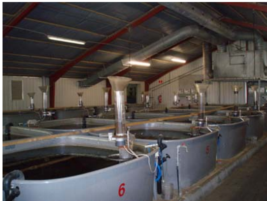
Figure 8.1 Inside Billund Aquaculture's eel farm. These 6000 litre tanks hold the glass eels and juveniles.
