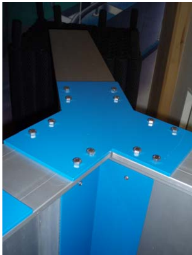
Figure 9.28 Detail of the junction plates between two Eco-Tanks
