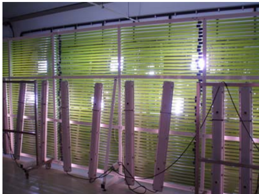
Figure 9.20 Part of their continuous culture system for microalgae.
