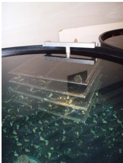
Figure 9.43 Tank surface area is increased by the addition of small shelves.
