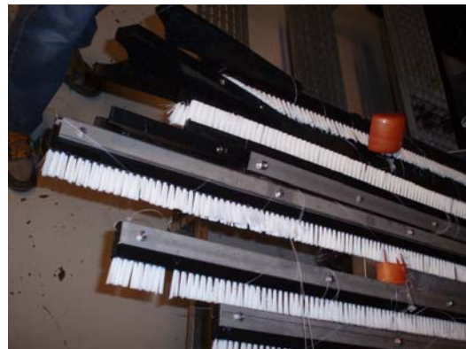
Figure 9.38 The brushes for the self cleaning tank system.
