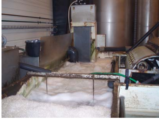
Figure 8.23 Foam fractionation in their homemade system. The horizontal approach.
